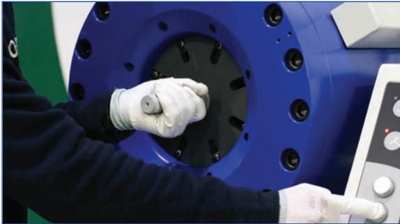
Master dies are guided through built-in channels on the tool on standard volume crimpers.
