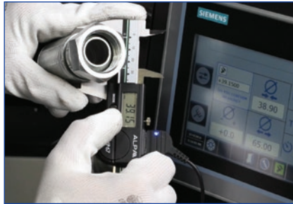
Digital Caliper automatically generates crimp correction for safety.
