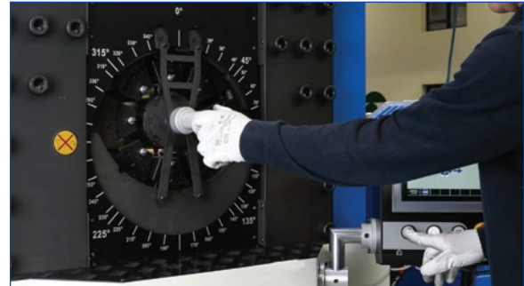
Tool held in place by built-in locking posts inserted into the crimper on high volume crimpers.
