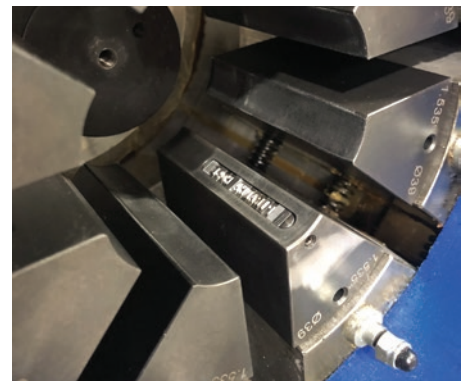
Marking Die Segments replace one of the eight standard die segments for that particular size (crimp diameter).
